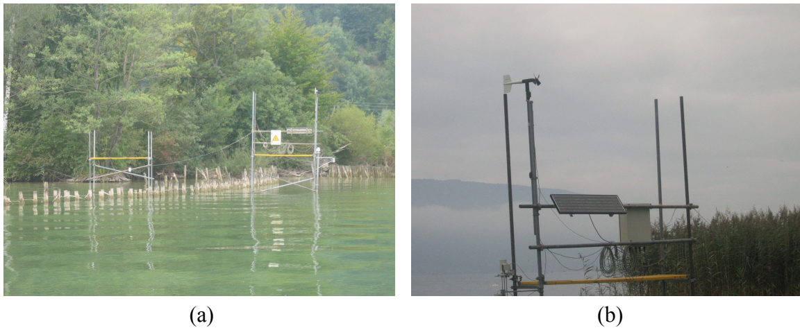
Fig. 3 (a) In situ wind and wave measurement platform at Lüscherz; (b) Wind anemometer powered by solar panels
