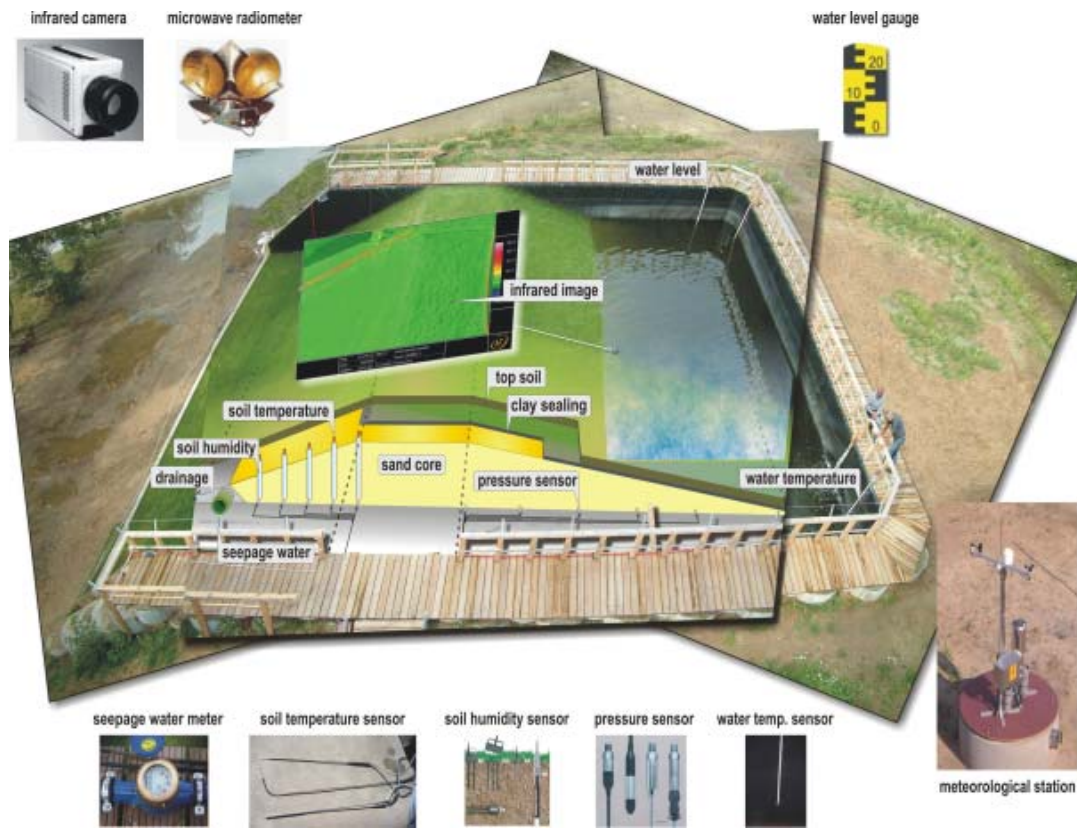
Figure 4. Open-air laboratory dike at the Franzius-Institut of the University of Hannover, in Hannover Marienwerder, Germany.
