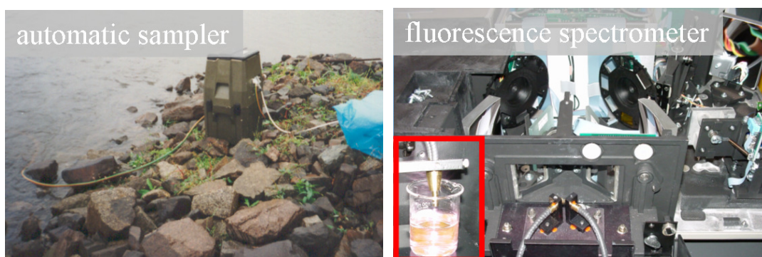
Figure 7 Sampling and ex-situ quantification of dye concentration.
