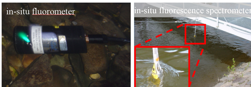
Figure 6 In-Situ measurements of dye concentration.
