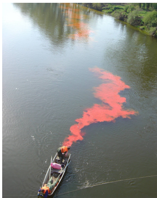
Figure 5 Input of the tracer Red Dye near Náměšice, Czech Republic
